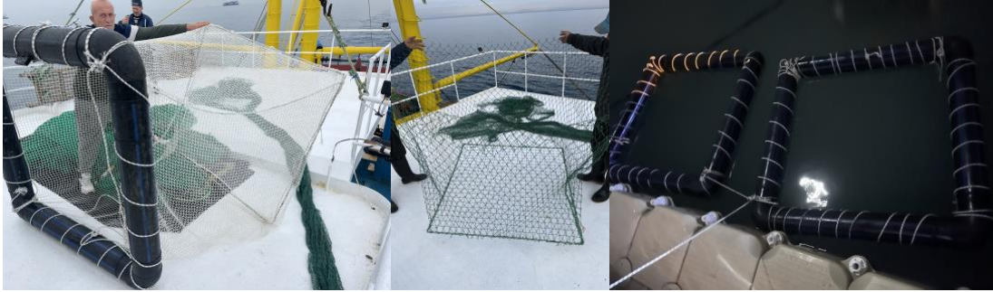
Figure 14. Experimental cages used for long-term survival trials (Left: Cage constructed with knotless polyamide (PA) netting (20 mm mesh). Middle: Cage constructed with knotted polypropylene (PP) netting (150 mm mesh). Right: Cages deployed at sea during the experiment.)
